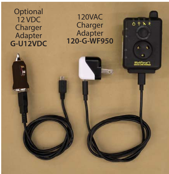
WorkForce® with Micro B USB Cord and 120VAC Charger Adapter (p/n: 120-G-WF950) Optional 12VDC Charger Adapter shown at left
