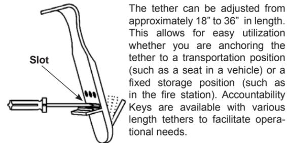
The tether can be adjusted from approximately 18" to 36" in length. This allows for easy utilization whether you are anchoring the tether to a transportation position (such as a seat in a vehicle) or a fixed storage position (such as in the fire station). Accountability Keys are available with various length tethers to facilitate operational needs.
