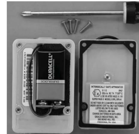
To change battery, remove the four screws securing the back cover. Remove back cover, disconnect and dispose of the exhausted battery and connect a new battery. Dispose of used batteries in accordance with national or local regulations.
