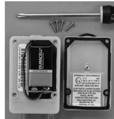
To change battery, remove the four screws securing the back cover. Remove back cover, disconnect and dispose of the exhausted battery and connect a new battery. Dispose of used batteries in accordance with national or local regulations.
